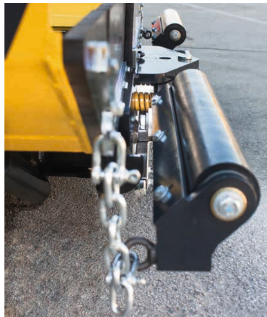
Impact-free docking – dampened bumper.
