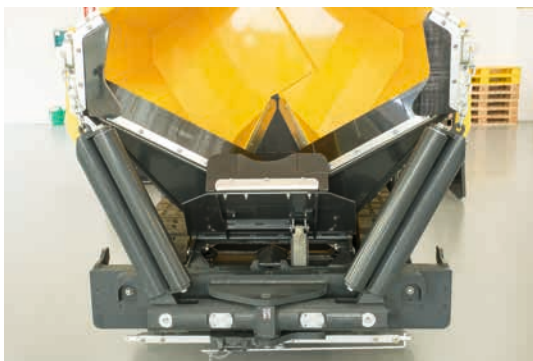
Hydraulic front gate – for a clean material flow.
