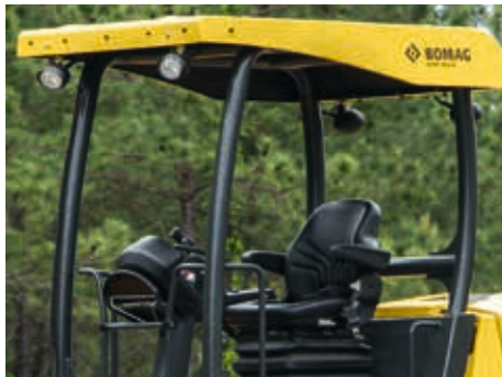
If no heating or air conditioning is required, the BW 11 RH-5 can also be delivered with ROPS/FOPS.
