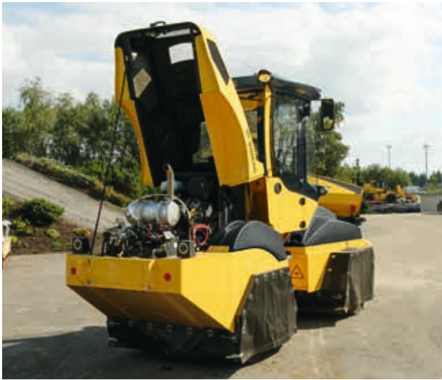
The hinged engine hood can be opened wide allowing fast, unobstructed access to the engine.
