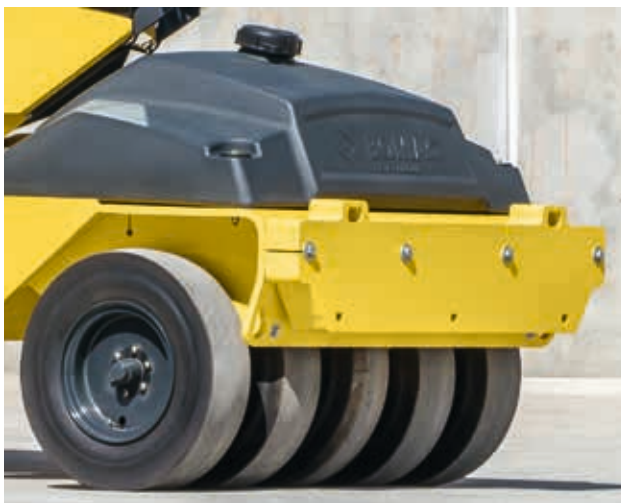
To increase stability the ballast compartments have been positioned extremely low down, as shown here above the front axle.
